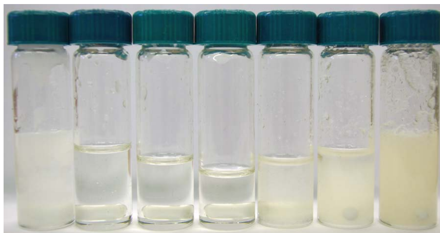
Figure 2. Melts of IA-CC with various molar ratios after cooling to room temperature, from left to right: 1 : 3, 1 : 2, 1 : 1.5, 1 : 1, 1.5 : 1, 2 : 1, 3 : 1. [Color figure can be viewed in the online issue, which is available at wileyonlinelibrary.com .]
